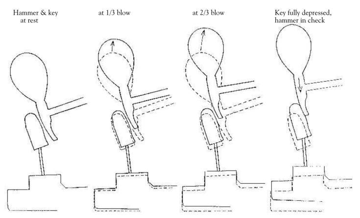
Note that the tail and backcheck pass with even clearance, and wedge tightly together with good contact area when in check
