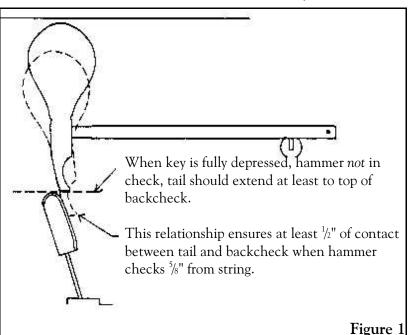
arc, and backcheck angle are correct then wear on backcheck leather is minimal because the contact area is large and the rubbing surfaces are smooth curves. *No "checkering" or extreme roughening of the tails will be necessary to achieve good checking*. Likewise, if tails etc. are *not* right then no amount of tail roughening will really give good results.
